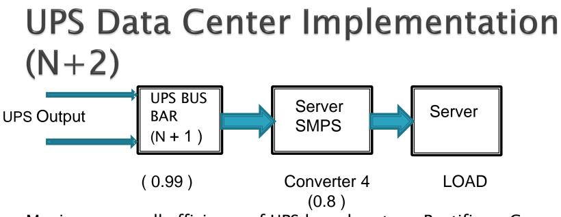
Maximum overall efficiency of UPS based system: Rectifier x Converter 1 x Converter 2 x Output Switch x Bus Bar x Converter  $4 = 0.99 \times 0.95 \times 0.95 \times 0.99 \times 0.8 = 0.70$
