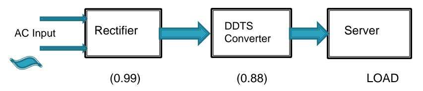
The optimum efficiency of a DDTS conversion system is: 0.99 x 0.88 = 0.87
